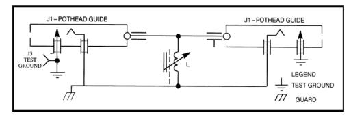
The simplified schematic diagram illustrates the Resonating Inductor. Note that the resonator electrically shunts the total specimen current; however, the measuring circuit is arranged to measure only the desired insulation current. The current taken by the Resonator is returned to its source without affecting these measurements.
