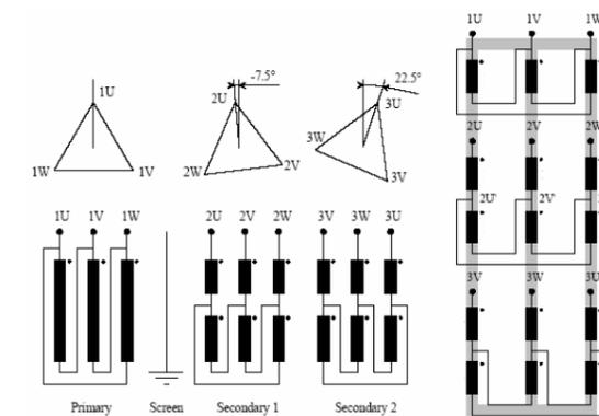
With the optional arbitrary phase shift software key (2293/ SKAP), the 2293 can measure turns and voltage ratio, phase displacement and excitation current of these special type transformers.
