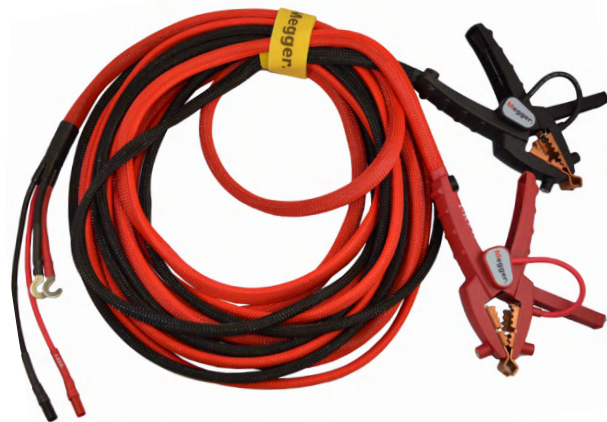
Universal Kelvin Clips make connections to transformers easy and secure, replacing the traditional two leads with one lead. Max opening: 4 in. (10 cm) Included: two banana plug inputs for lead connection to small specimens.
