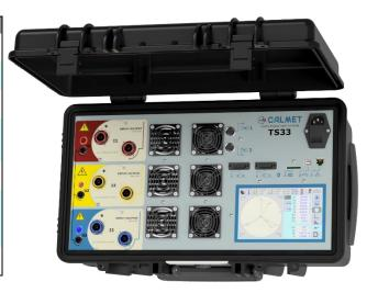
The Calmet TS33 portable test system consists of a three-phase reference meter of accuracy class 0.05% (or 0.1%) and an integrated three-phase current and voltage source up to 3x120A/600V. The TS33 is designed for analysis of complete metering installations and local mains conditions.
