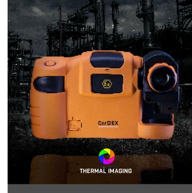
The **TC7000** Thermal Imaging Camera is a proven tool for predictive maintenance; however thermography in hazardous (explosive) areas has not been easily accessible due to certification restrictions.
