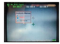
The analysis menu is split into two sections; Spots and Isotherms. Selecting Spots enables live spot measurement mode with three options.
