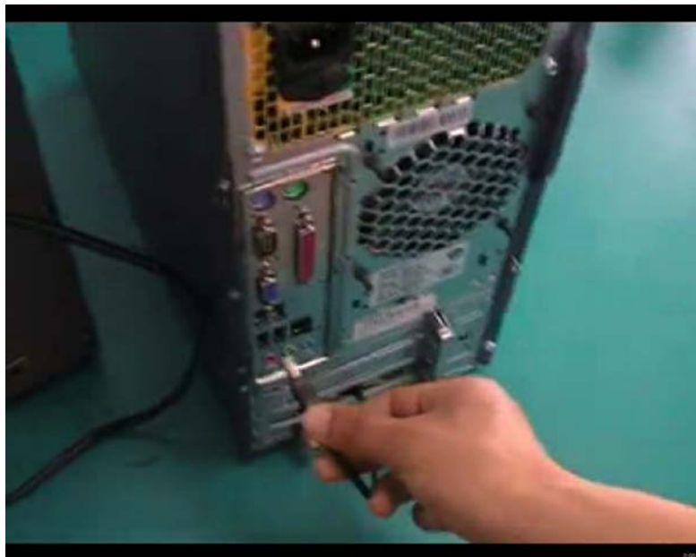
Fig 2 Connect USB cable of 1801A card to USB interface of PC.
