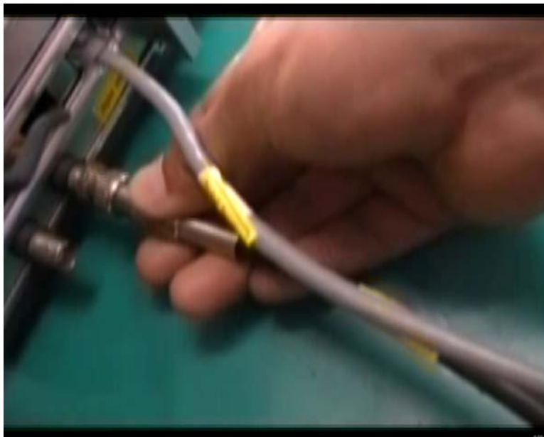
Fig 7 Connect “Visual Video 1” connector onto corresponding interface “Visual Video” on PC
