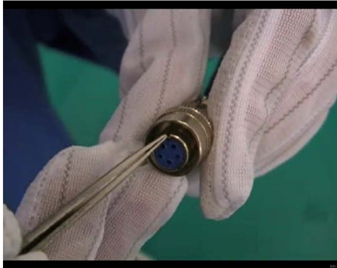
Fig 2. Please notice there is a small gap on the sensor connector, which needs to be aimed at the gap in “Sensor” on the camera body.
