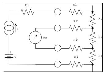
From a voltage source U, a generator supplies a current of value I and determined waveform (pulse, alternate or direct)
