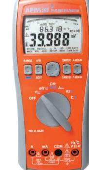
100,000/10,000 count extra large digital display 43 segments analog bar graph Auto Backlit, Dual display Auto AC, DC and AC+DC on Voltage & Current mode with Frequency indication Auto selection on Ohm, Diode or Continuity On-Screen-Menu Selection Navigator Key Drive High Frequency Rejection (HFR) 0.015% DCV accuracy AC+DC True RMS indication 0.5 ms Peak Hold Auto Hold Store/Recall memories dBm/dB measurement 20000 records data logging capacity
