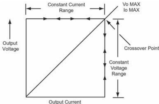
Figure 4 – CC/CV Characteristic
