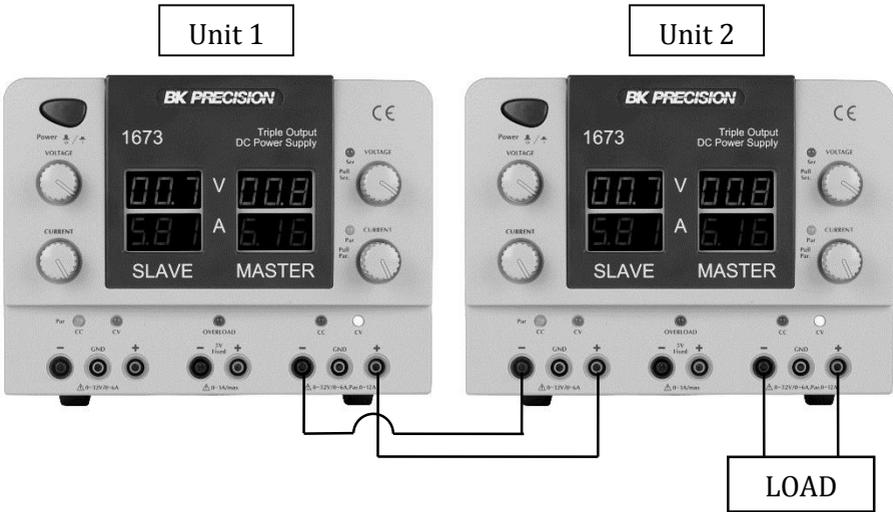
**Figure 8 – Connecting Multiple Units in Parallel**
