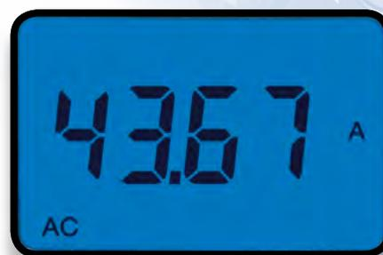
2. Start **True InRush** acquisition. The clamp then displays the trigger threshold and begins the monitoring phase.
