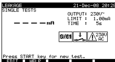
Differential leakage current menu
