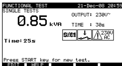
Example of apparent power measurement result
