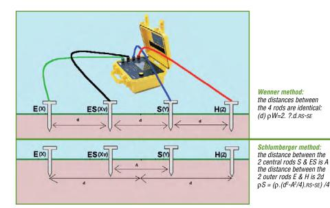
When it is possible to choose the position of the earth connection, resistivity measurements can be used to check the soil and determine where the earth resistance will be lowest (optimization of building costs).
