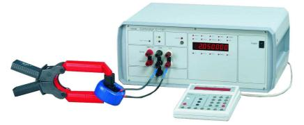
C101FB and C101FC Calibrators have increased output power to control the coils in order to check clamps and clamp meters up to 1000A DC and AC.
