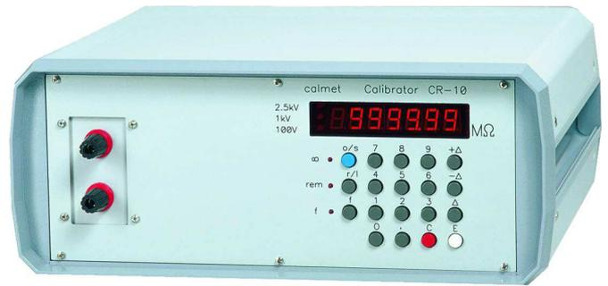
The CR10 Calibrator is used for testing of analogue and digital insulation meters. CR10 reproduces resistance in range 10kΩ...10GΩ with resolution of 10kΩ (6 decades of setting resistance) at working voltages up to 2500V.
