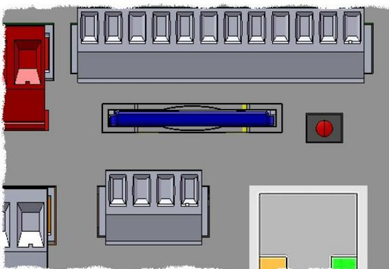
The red LED of the key located next to the SD card signals that the logger is active. During writing to the card the LED becomes dark for a short time.
