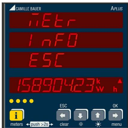
**Meter reading:** By pressing the key **i** for a longer time an operating mode is started, which allows to read all the meter contents via line 4. This mode is automatically stopped after 30s without any key pressed or via the key **ESC**. If this mode is active no measurement info is displayed on line 1 to 3.
