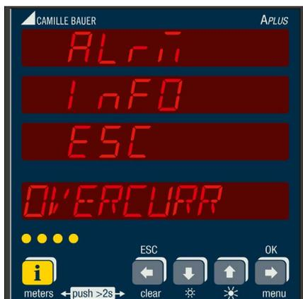
**Alarm display:** By shortly pressing the key **i** an operating mode is started, which allows to display alarm state texts and to acknowledge alarms via line 4. If there are no configured alarms the message "No LED used" is displayed and then the mode is stopped. Otherwise the mode is automatically stopped after 30s without any key pressed or via the key **ESC**. If this mode is active no measurement info is displayed on line 1 to 3.
