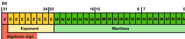
The first register contains Bits 15 – 0 of the 32-bit number (bit 0...15 of the mantissa).
