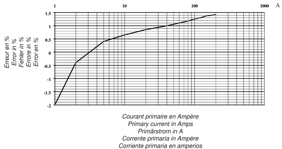
■ **Calibre 1000 A (1 mV/A) / Range 1000 A (1 mV/A) / Bereich 1000 A (1 mV/A) /
