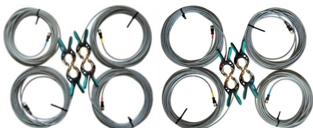
H winding test cable set
