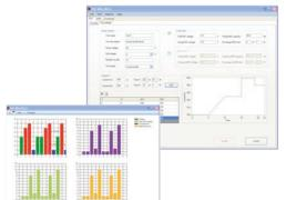
the current, voltage and capacity values as well as the waveforms can be observed. Additionally, online tracking function using histogram shows the distribution of the voltage on each cell of the battery string.
