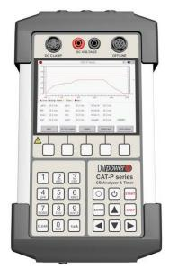
Handheld Circuit Breaker Analyzer & Timer CAT-P is a digital instrument for circuit breakers condition assessment. CAT-P records timing graphs of main contacts, DC substation battery voltage, Trip and Close coil currents. Main contacts operating time in on-line mode is calculated based on AC secondary CT's currents. The timing channels record closing and opening of the main contacts.
