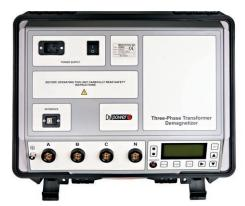
The Three-Phase Transformer Demagnetizer DEM60C is a portable instrument designed for a single and three-phase transformer core demagnetization. Demagnetization process eliminates the remanent magnetism from the transformer core. In this way users avoid problems such as high inrush currents at the start-up of power transformers, incorrect operation of protective relays, erroneous diagnostics or inaccurate measurement on a transformer.
