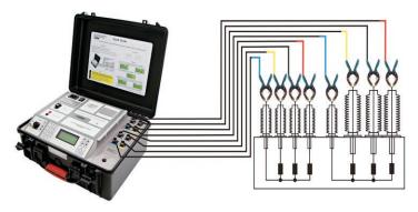
Using two sets of four cables, all bushings of HV and LV sides are connected at once. The connection to the transformer is made with two-contact clamps providing for four-wire Kelvin test method.
