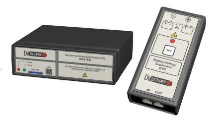
It can be used during a battery charging/discharging process, as well. If used in a combination with the BLU device, the user can perform additional tests: measurements of a battery internal and intercell connection resistances as well as a short circuit current estimation.
