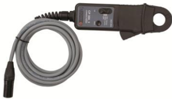
Current clamp 30/300 A with extension 5 m (16.4 ft)
