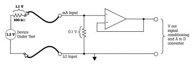
Figure 1. Circuitry of a shunt multimeter used as an ammeter.
