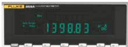
The Fluke 8808A includes two low impedance low current ranges for measuring sensitive leakage currents
