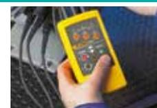
Check the correct rotation of motors prior to connection.
