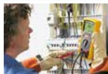
Insulation test at a distribution panel
