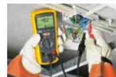
Wiring test in a small distribution box – all in one spot
