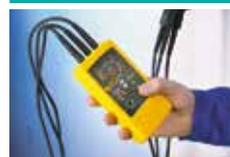
Determine the presence of phase sequence of multiphase electrical supplies.
