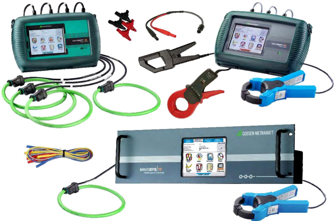
There are many possible current probe options available from Gossen Metrawatt to fulfill your current measurement requirements for both MAVOWATT and MAVOSYS instruments. Many of these current probes connect directly into the MAVOWATT 20/30/40/70 and MAVOSYS 10. For the MAVOSYS 10 a 61MAC input module allows connection of the available current probes to the instrument.
