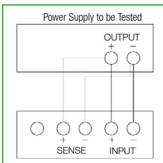
Remote sensor connector sockets and trigger connector socket are included. The instrument is automatically switched to sensing mode operation as soon as the remote sensors are connected.
