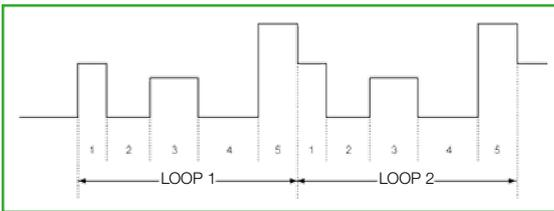
Extensive sequential test functions with 10  $\mu$ s as the smallest step rate and 100,000 s as the largest step rate. Cyclical addresses can be freely selected and one sequence can be combined with another, in order to execute even more complex test procedures.
