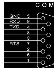
The cable with the designation Z5232 000 R0001 must be used for connecting a PC or a terminal.
