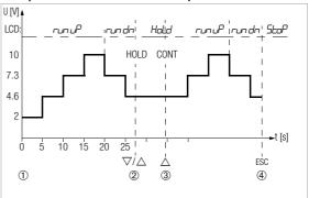
**Interval parameters:** output quantity: U (range of  $0 \dots 15$  V), SER-L = 2 V, End = 10 V, number of interval SEEP5 = 3, L = 5 s, RadE = RaLa
