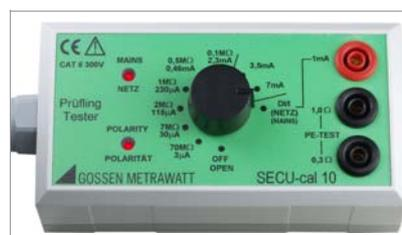
The calibration adapter is used for testing the measuring safety of test and measuring instruments by measuring protective conductor resistance, insulation resistance and leakage current.
