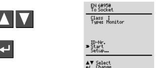
This is the default setting. Refer to chapter 7 on page 17 for other types of connection. If the DUT has been connected to the test socket, safety class recognition is performed (SC I or SC II). Otherwise, the safety class must be specified manually.
