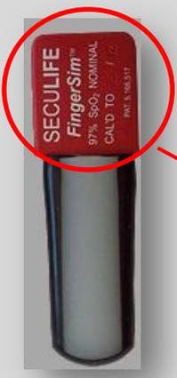
2.) Checking the SpO2 function with the "SECULIFE pulse oximeter module" The nominal value of the FingerSim™ (here: 97 %) should approximately correspond to the value displayed at the DUT (here: 98 %).
