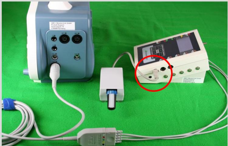
1.) Connection for SpO2 measurement a connection is established between SECULIFE NIBP and the holder via a 7 pin mini-DIN cable.
