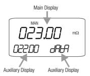
The main display appears immediately after the milliohmmeter is switched on, but the auxiliary displays have to be activated by pressing the DATAI CLEAR key.
