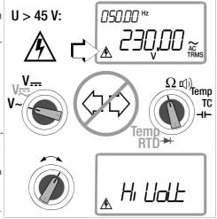
ment is disabled. The measuring function is not switched until dangerous touch voltage is no longer applied to the input. If the instrument switches itself off in the event that hazardous touch voltage is applied (during memory mode operation with large
