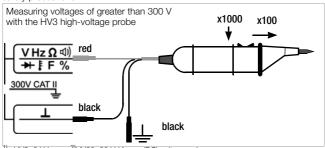
1) HV3: 3 kV <sup>2)</sup>HV30: 30 kV for --- (DC) voltage only
