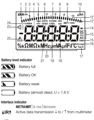
IR IR interface in stand-by mode (ready to receive starting commands)
