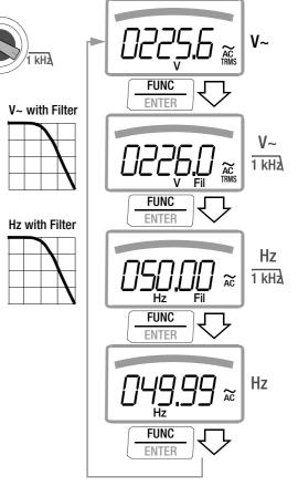
5.1.3 Alternating Voltage and Frequency Measurement V AC and Hz with Selectable Low-Pass Filter (METRAHIT X-TRA OUTDOOR TECH PRO ONIV)
