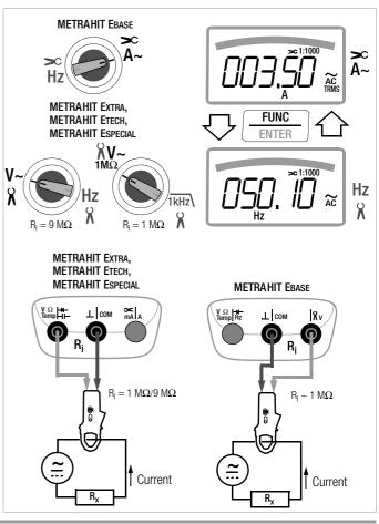
5.7.5 Direct, Pulsating and Current Measurement with Current Clamps Transformer A DC, A (DC+AC), A AC and Hz (METRAHIT EXTRA, METRAHIT ETECH and METRAHIT ESPECIAL ONIY)
