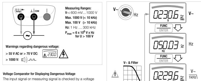
The input signal or measuring signal is checked by a voltage comparator for dangerous spikes, because these do not appear at the display when the low-pass filter is used.
