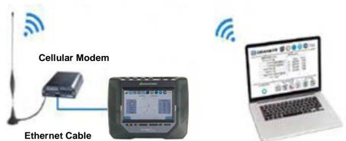
**Figure 1. Typical Wireless Modem Application**
