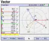
Depending upon the measured quantity and the measuring range, numeric measured values are displayed as 2 to 4-digit figures with floating decimal point, unit of measure and preceding minus sign if applicable. The read-out of measured values takes the selected transformation ratios of the utilized current and voltage transformers into consideration.
