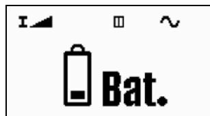
Figure 3.9: Battery Status After Pressing the START Key
