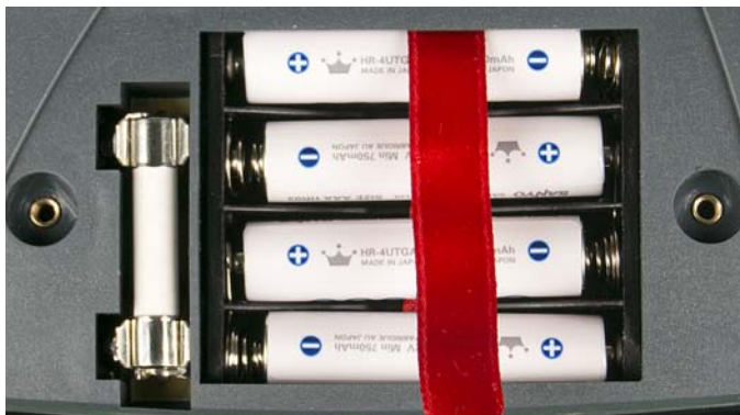
Figure 5: Correct Battery Polarity
