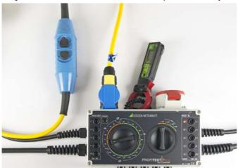
Documentation of protective conductor resistance and insulation resistance measurements with the help of the PROFITEST MXTRA as an accessory
