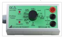
The calibration adapter is used for testing the measuring accuracy of test instruments in accordance with DIN VDE 0701/0702/0751. To meet the requirements set forth by accident prevention regulation DGUV provi-
