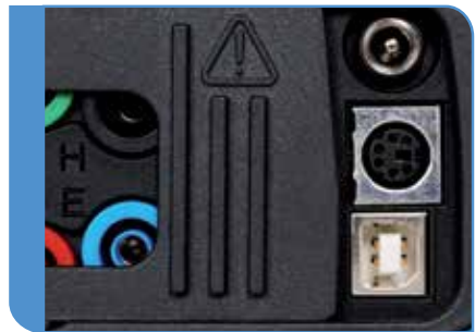
USB and RS232 communication ports.
