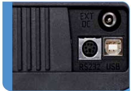
USB and RS232 communication ports.
