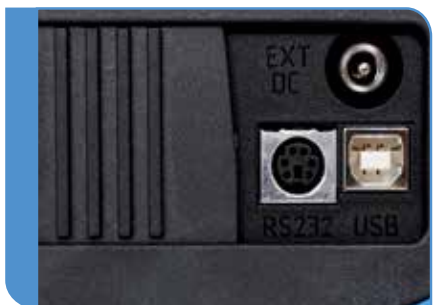
USB and RS232 communication ports.
