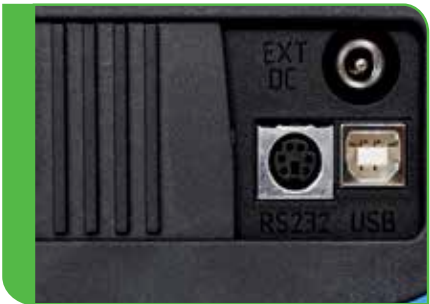
USB and RS232 communication ports.
