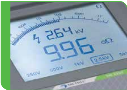
Large analogue / digital LCD with backlight
