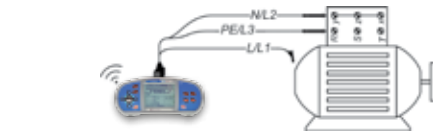
Test circuit for continuous resistance measurement
