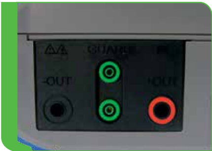
Guard terminal for connecting shielded test leads
