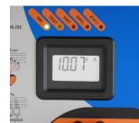
**10.** Impedance measurement with a Resolution of  $1 \text{ m}\Omega$ ...
