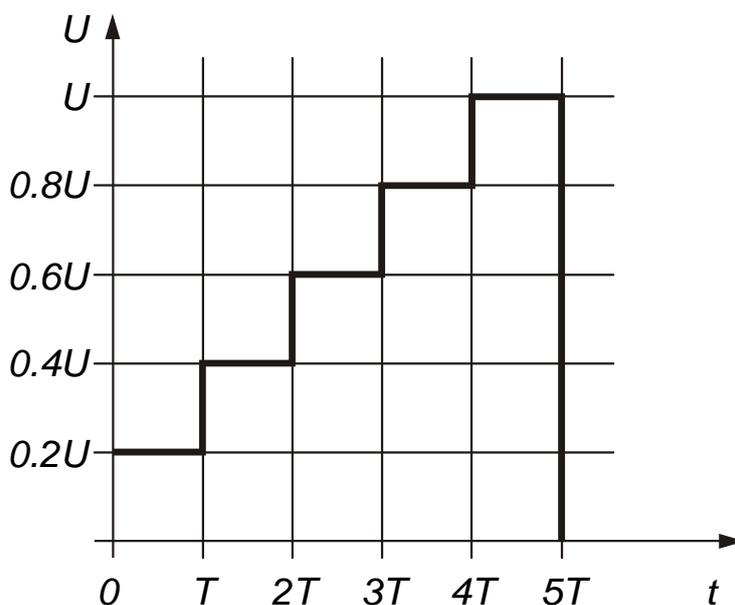
**Fig. 23.** Step-up test voltage
