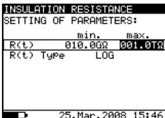
**Fig. 14 .** Set-up menu of the Graph R(t)
