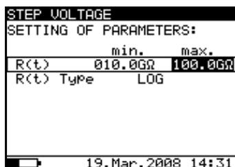
**Fig. 26.** Set-up menu of the Graph  $R(t)$
