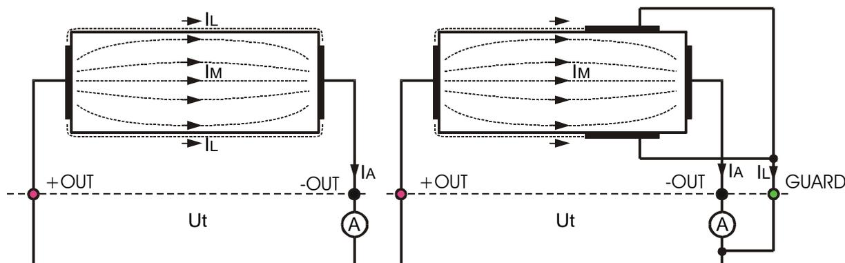
**Fig. 8.** Connection of GUARD terminal to measured object
