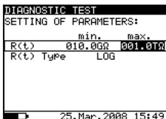
**Fig. 20.** Set-up menu of the Graph R(t)
