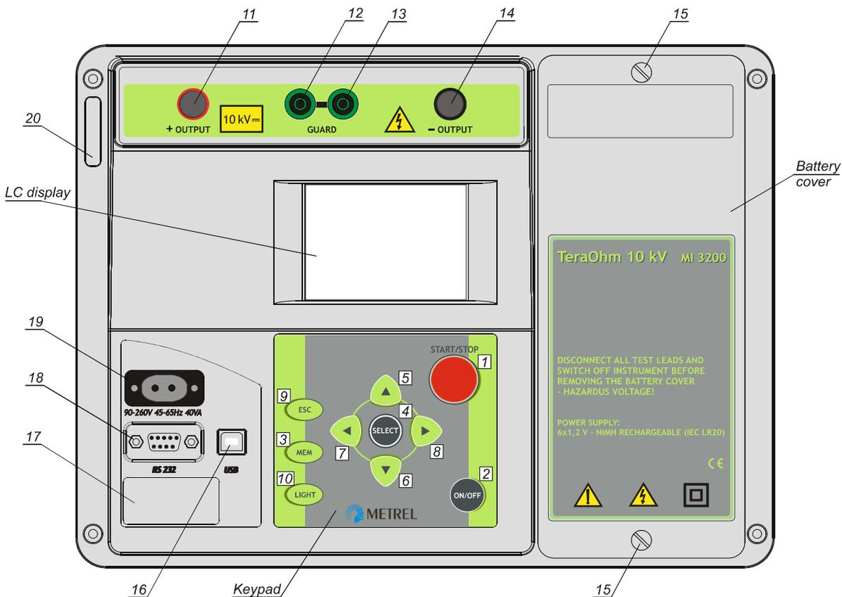
**Fig. 1. Front panel**
