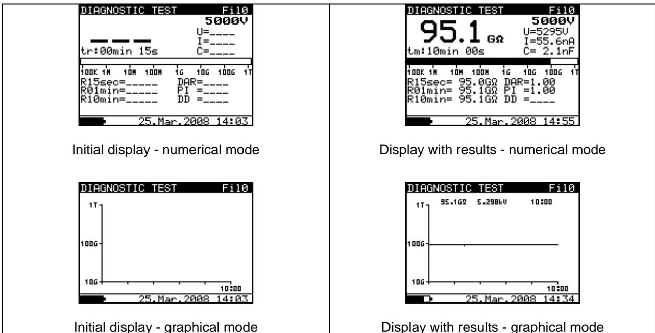
**Fig. 16. Diagnostic test display states - Graph R(t) enabled**
