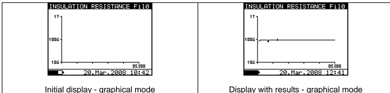
**Fig. 11. Insulation Resistance function display states - Graph R(t) enabled**
