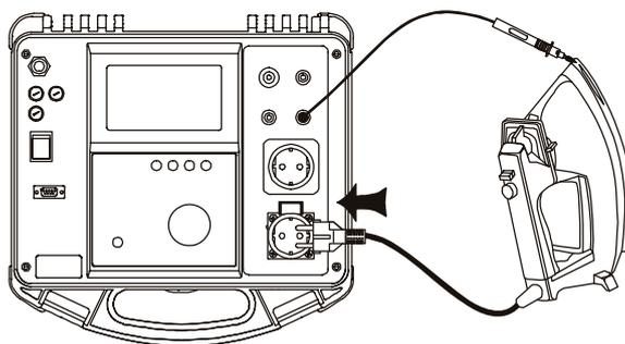
Fig. 35. Connection of CLASS I equipment
