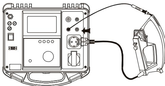
Fig. 57. Connection of CLASS I equipment
