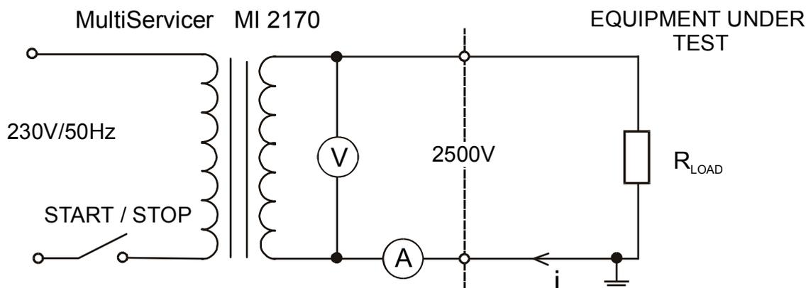
Fig. 2. Test circuitry
