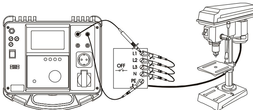
Fig. 7. Connection of test leads
