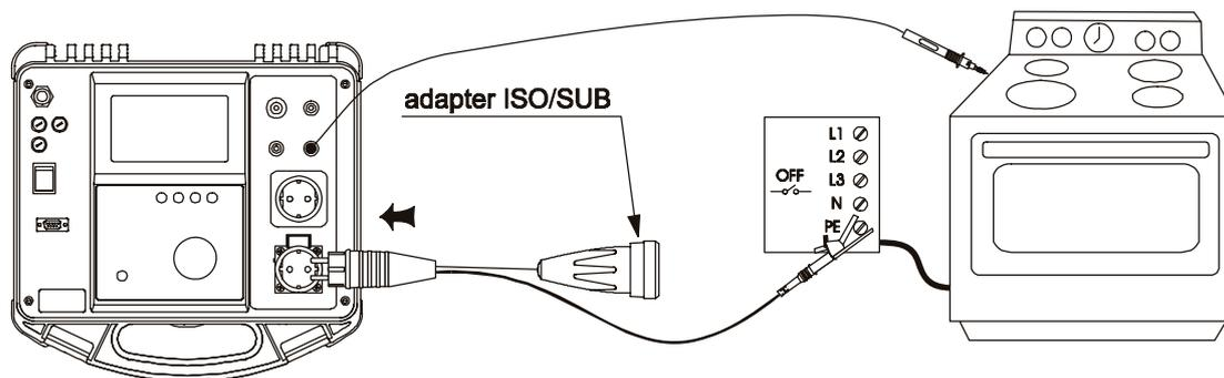
Fig. 37. Connection of hard-wired equipment
