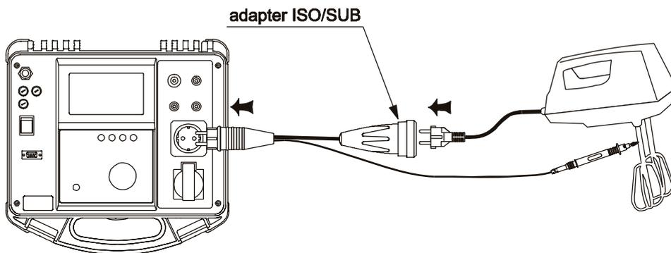
*Fig. 46. Connection of CLASS II equipment*
