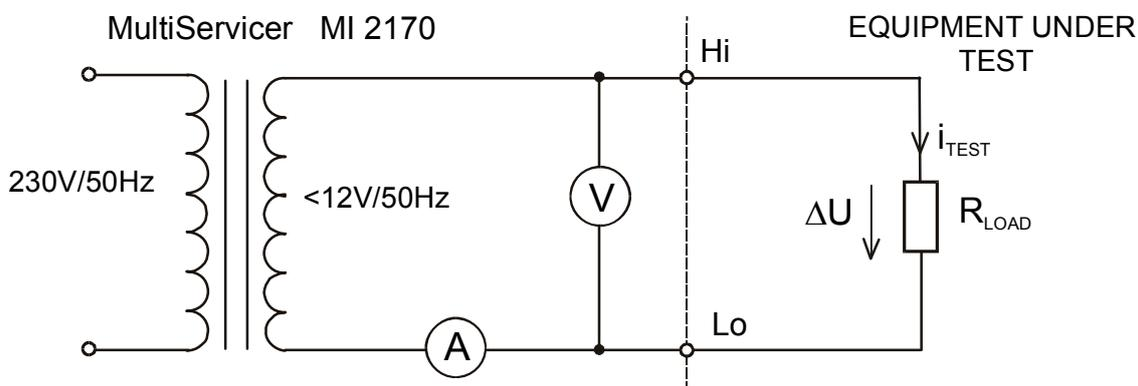
Fig. 11. Test circuitry
