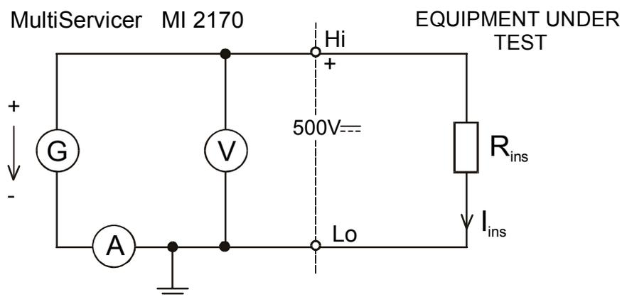
Fig. 8. Test circuitry
