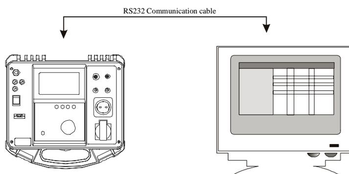
Fig. 63. Connection of MultiServicer to PC (9 or 25 pin connector)
