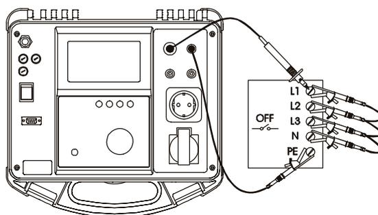
*Fig. 4. Connection of test leads*
