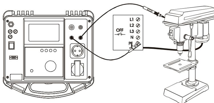
Fig. 15. Connection of test leads
