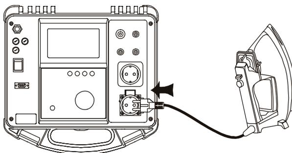
Fig. 31. Connection of CLASS I equipment
