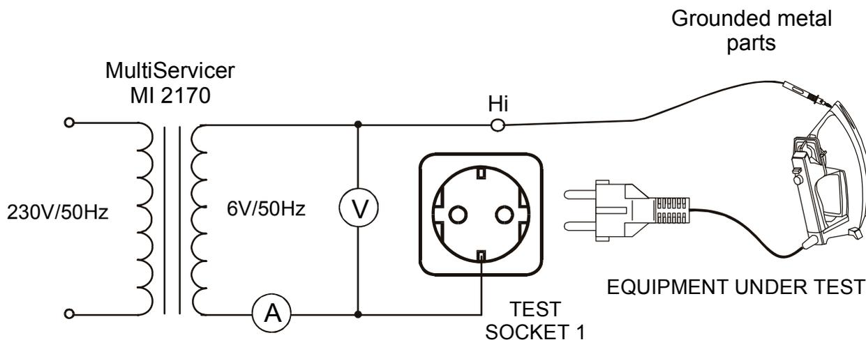
Fig. 53. Test circuitry
