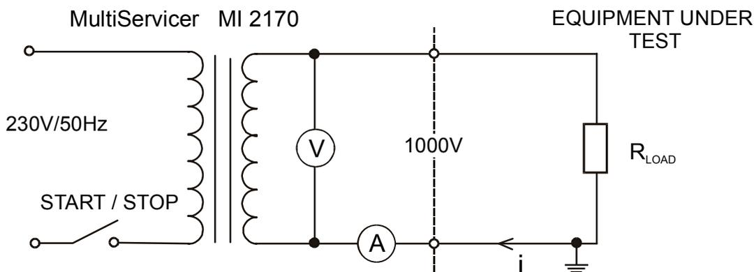
Fig. 5. Test circuitry
