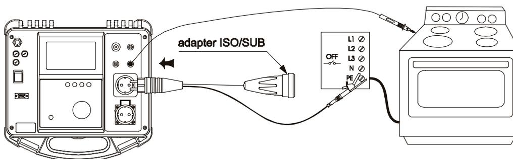
Fig. 58. Connection of hard-wired equipment
