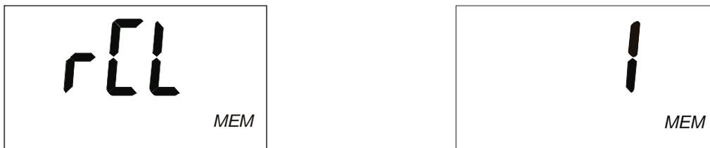
Fig. 61. Entering the recalling mode, offered group for recalling results
