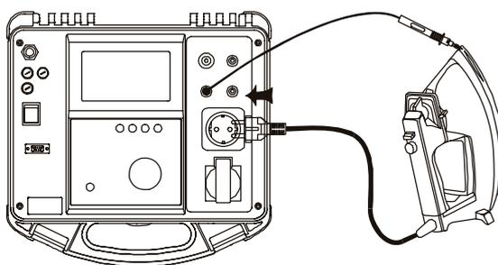
Fig. 51. Connection of CLASS I equipment
