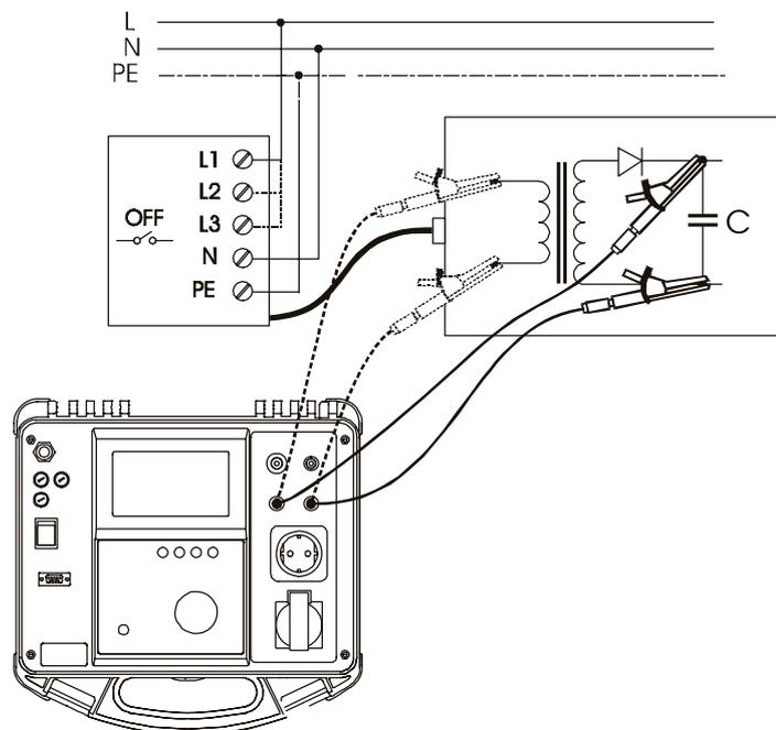
Fig. 24. Connection of test cable
