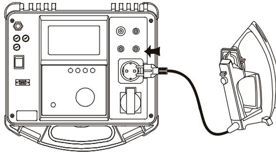
*Fig. 45. Connection of CLASS I equipment*
