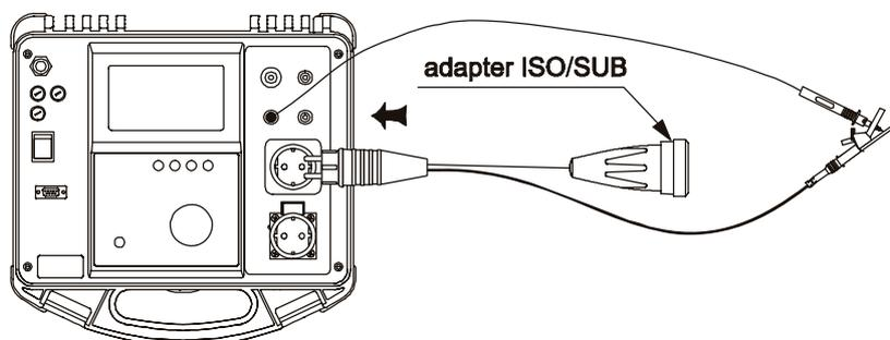
Fig. 50. Zero calibration
