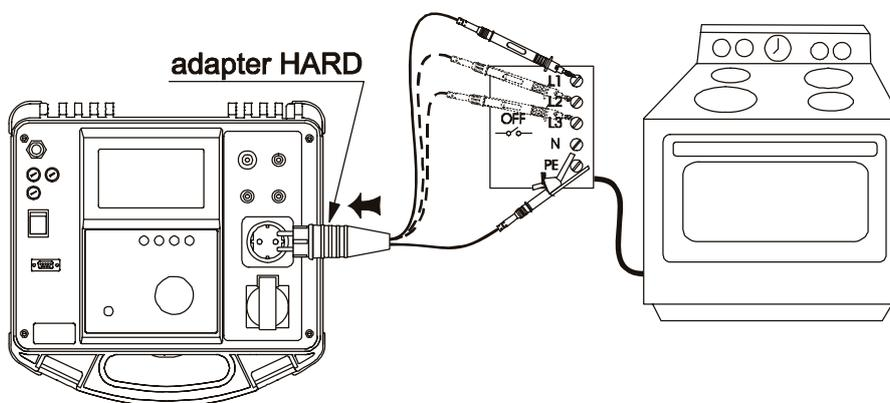
*Fig. 47. Connection of hard-wired equipment*
