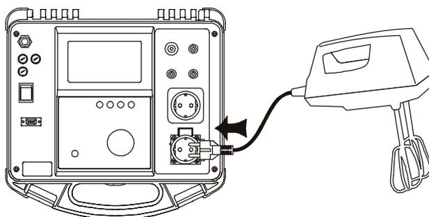
Fig. 28. Connection of CLASS II equipment
