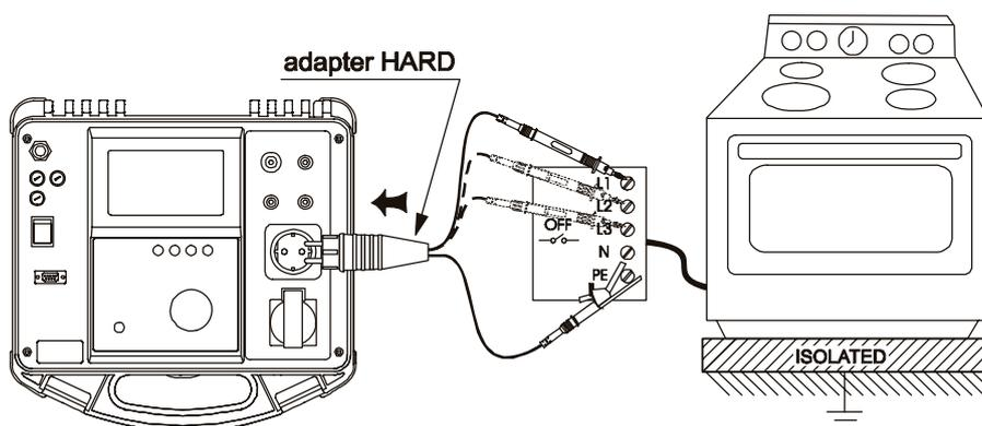
Fig. 42. Connection of hard-wired equipment
