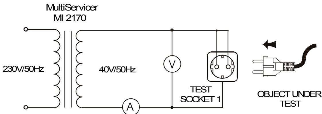
Fig. 38. Test circuitry
