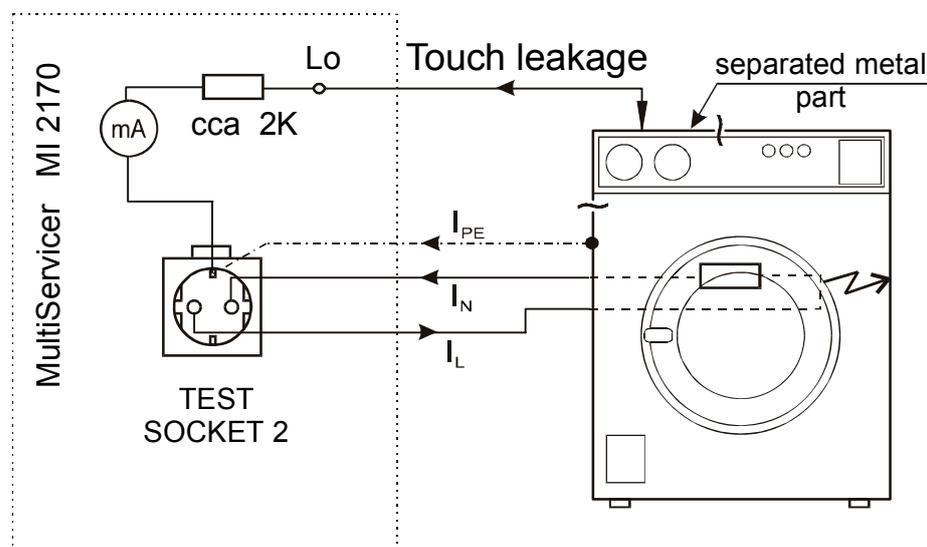
Fig. 33. Test circuitry
