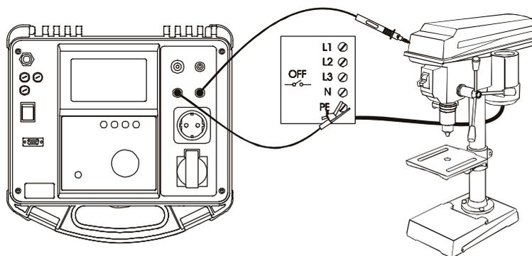
*Fig. 20. Connection of test leads*
