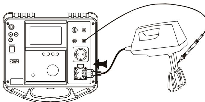
Fig. 36. Connection of CLASS II equipment
