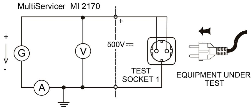
Fig. 43. Test circuitry
