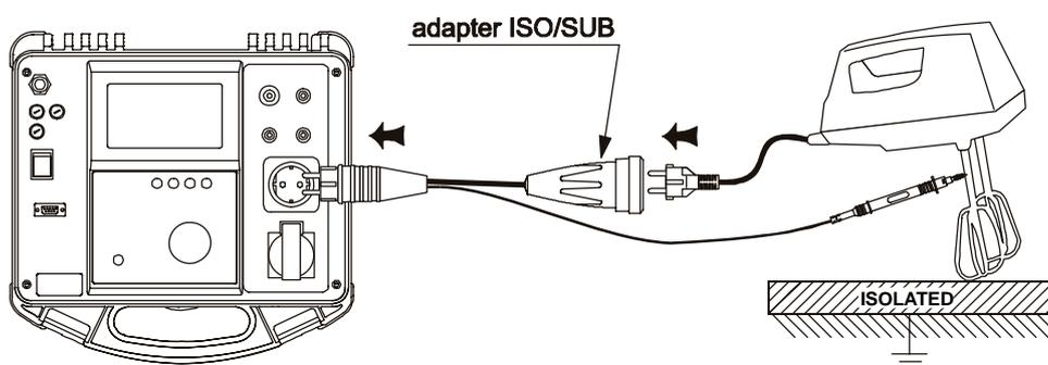
Fig. 41. Connection of CLASS II equipment
