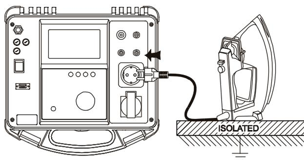
Fig. 40. Connection of CLASS I equipment
