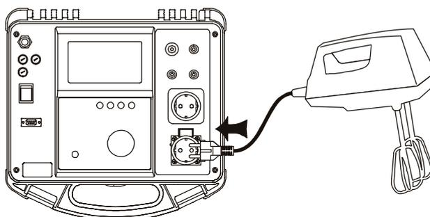
Fig. 32. Connection of CLASS II equipment
