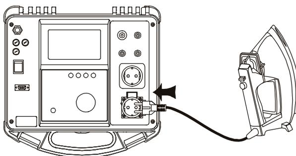
Fig. 27. Connection of CLASS I equipment
