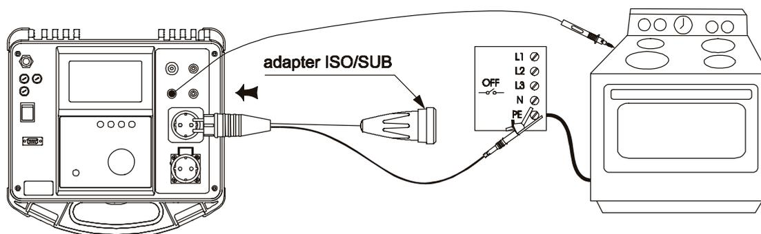
Fig. 52. Connection of hard-wired equipment
