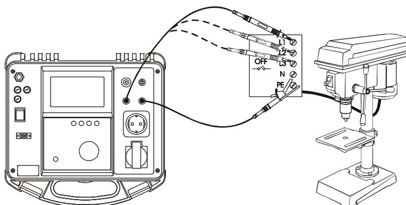
Fig. 10. Connection of test leads
