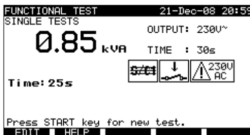
Example of apparent power measurement result
