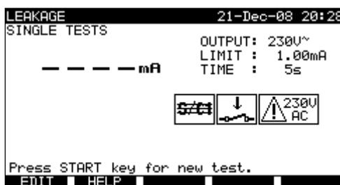
Differential leakage current menu
