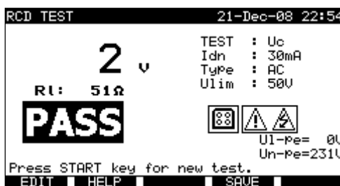
Example of contact voltage measurement results
