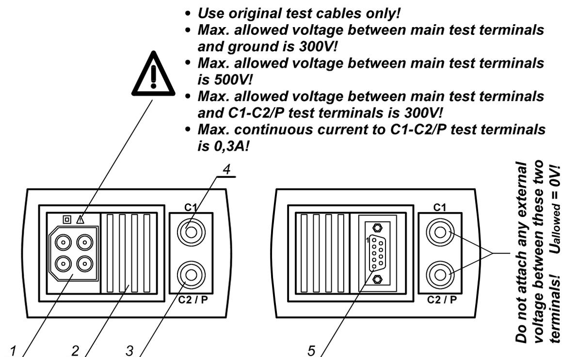
**Fig. 2.** Connector panel
