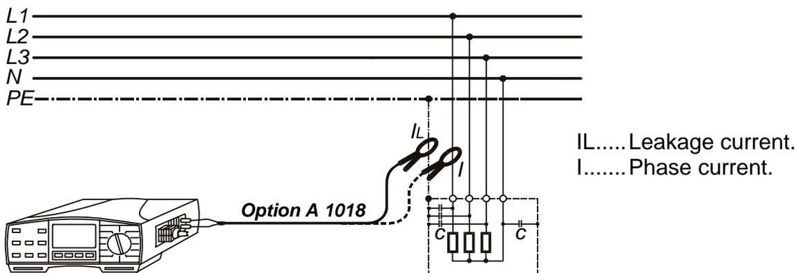
Fig. 76. Connection of optional Low-range Current Clamp (Order No. A 1018)
