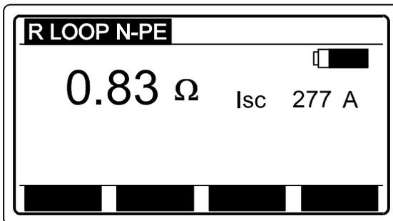
$$I_{psc} \text{ (Isc marked on display)} = \\ = U_n \cdot 1,06 / R_{LOOP N-PE}$$
