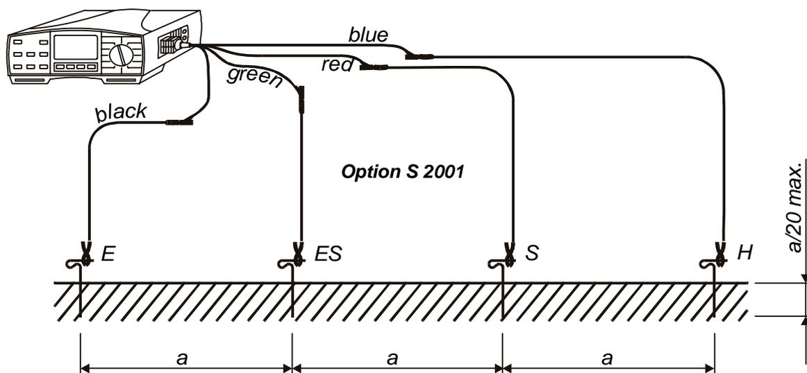
Fig. 36. Connection of optional Earth Test Set – 20 m (Order No. S 2001)
