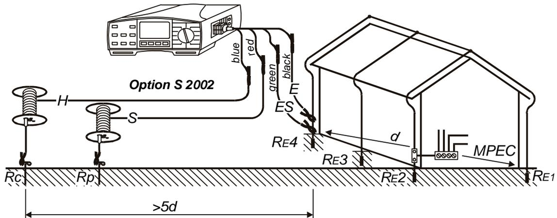
Fig. 26. Connection of optional Earth Test Set – 50 m (Order No. S 2002)
