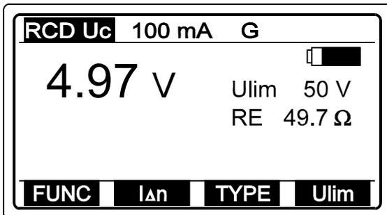
RE (Earth Resistance) is displayed meaning auxiliary test probe has been used. In that case Uc is measured with respect to auxiliary test probe (real ground).
