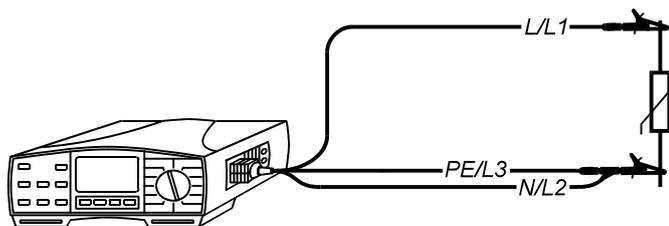
**Fig. 10.** Connection of tested device
