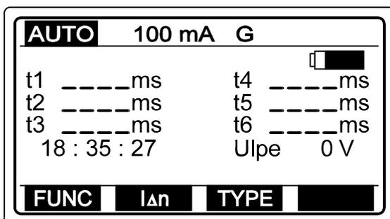
t1 to t6 ...Trip out time of each partial test.
