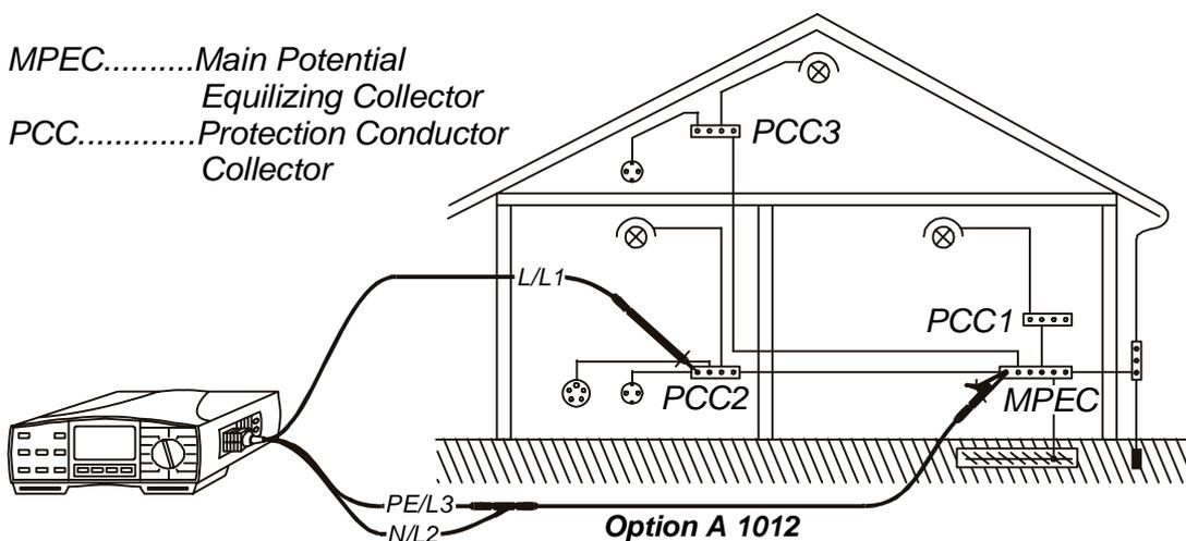
**Fig. 15.** Connection of Universal Test Cable and optional Probe Test Lead (Order No. **A 1012**)
