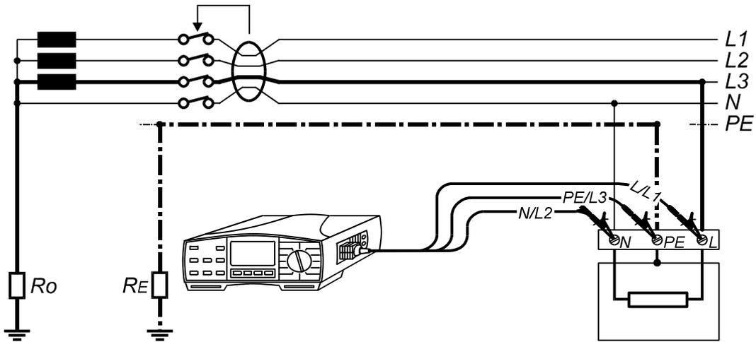
Fig. 60. Connection of Universal Test Cable
