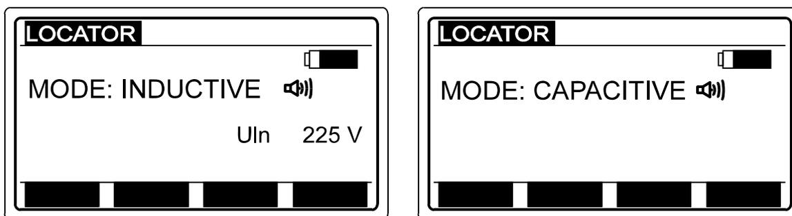
**Fig. 88.** Display menu, while tracing function is running - installation under mains voltage (left figure) and voltage-free installation (right figure)
