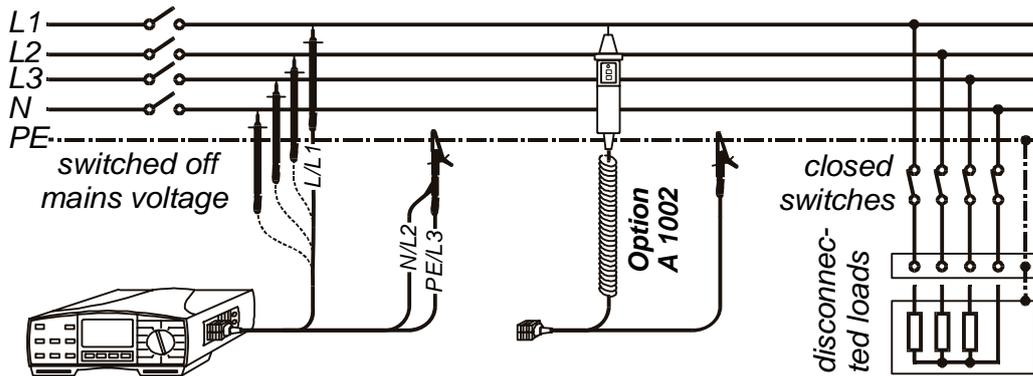
**Fig. 6.** Connection of Universal Test Cable and optional Tip Commander (Order No. A 1002)
