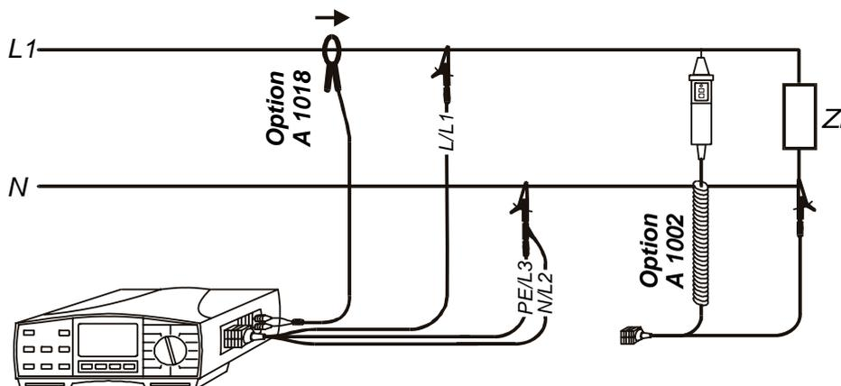
**Fig. 90.** Connection of optional Low-range Current Clamp (Order No. A 1018) in combination with Universal Test Cable or opt. Tip Commander (Order No. A 1002)
