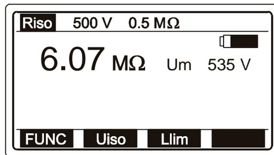
**Fig. 7.** Example of Insulation resistance test result
