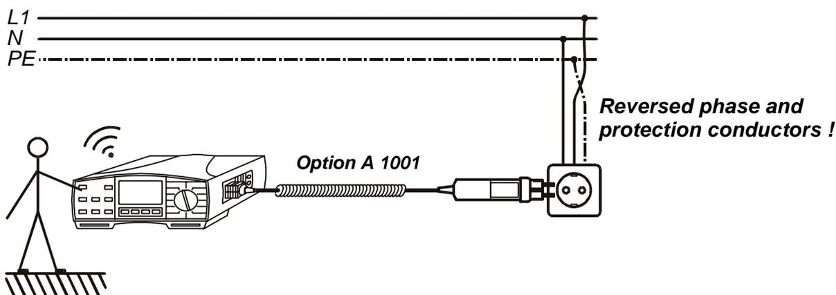
**Fig. 38.** Connection of optional Plug Commander (Order No A 1001) to mains outlet with reversed L and PE conductors
