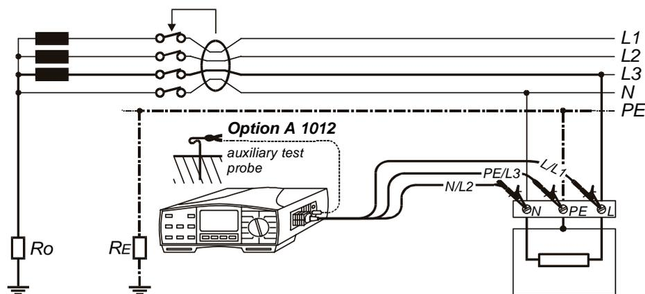
**Fig. 42.** Connection of Universal Test Cable, measurement with or without auxiliary test probe connected via optional Probe Test Lead (Order No. A 1012)
