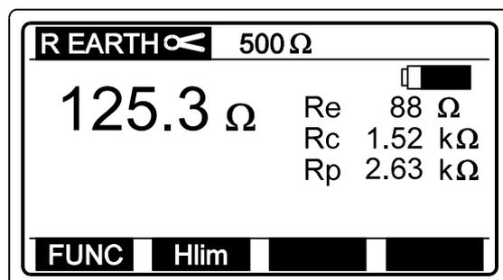
*Fig. 30. Example of Earth Resistance test result*
