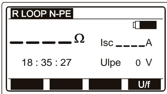
Isc ..... Prospective short-circuit current in fault loop, between phase and protective terminals.
