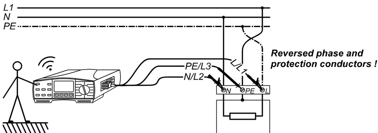
**Fig. 39.** Connection of Universal Test Cable to load connection terminals with reversed L and PE conductors
