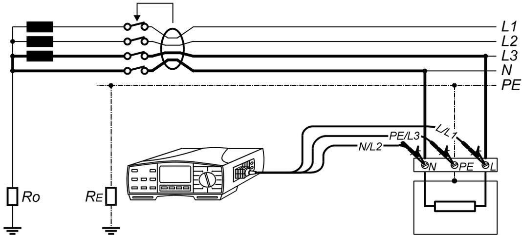
**Fig. 66.** Connection of Universal Test Cable
