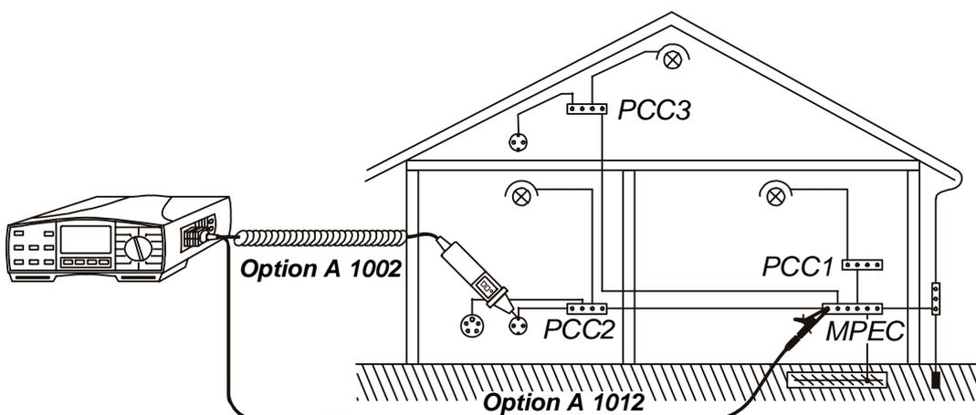
**Fig. 16.** Connection of optional Tip Commander (Order No. **A 1002**) and optional Probe Test Lead (Order No. **A 1012**)
