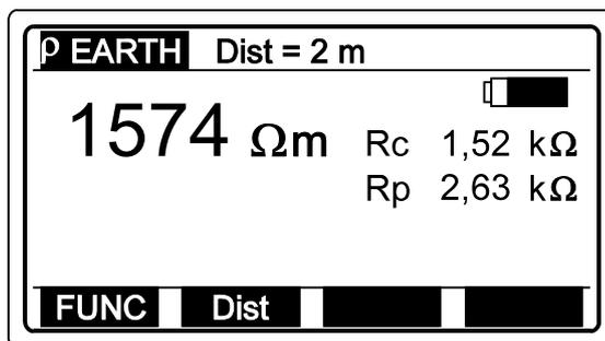
*Fig. 37. Example of Earth Resistivity test result*
