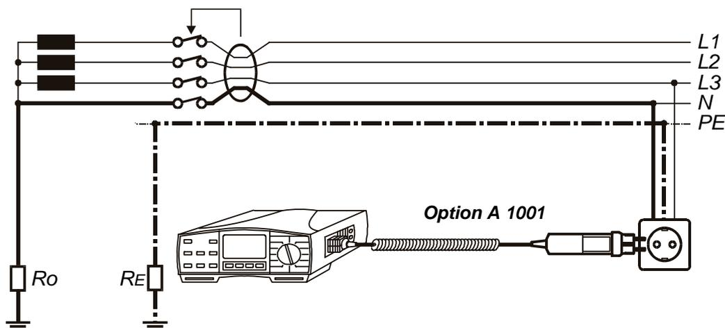
**Fig. 69.** Connection of optional Plug Commander (Order No. A 1001)
