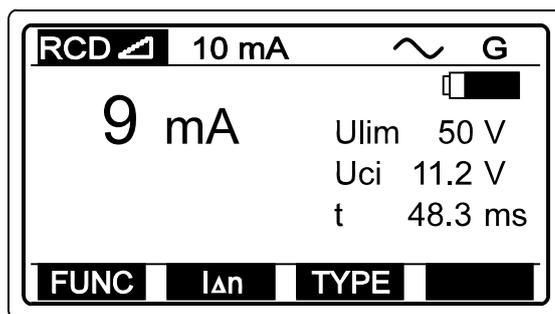
*Fig. 50. Example of Tripping current test result*
