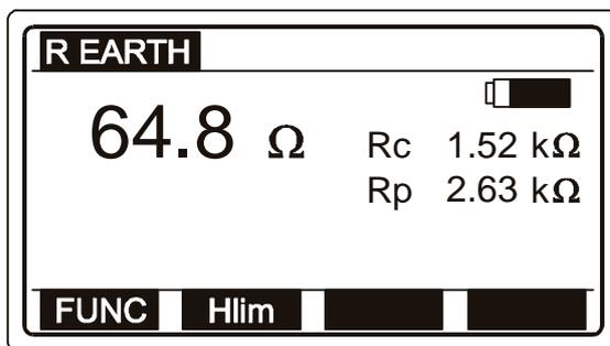
Both resistances, Rc and Rp are measured and displayed continuously.
