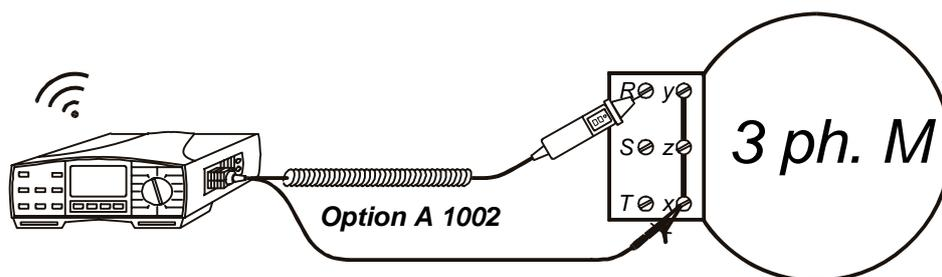
**Fig. 21.** Connection of optional Tip Commander (Order No. A 1002)
