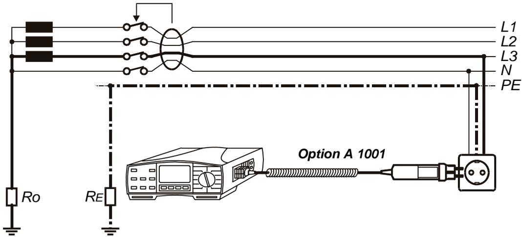
Fig. 59. Connection of optional Plug Commander (Order No. A 1001)
