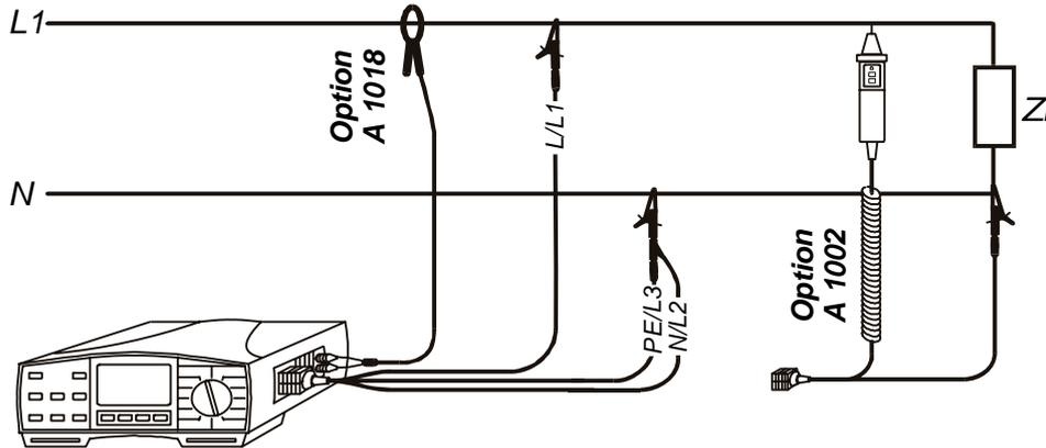
**Fig. 95.** Connection of optional Low-range Current Clamp (Order No. A 1018) in combination with Universal Test Cable or opt. Tip Commander (Order No. A 1002)
