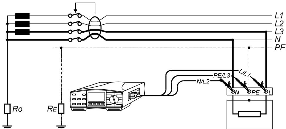
Fig. 70. Connection of Universal Test Cable
