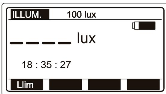
*Fig. 81. Illumination measurement initial menu*
