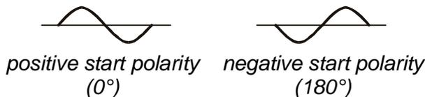
**Fig. 47.** Start polarity of test current
