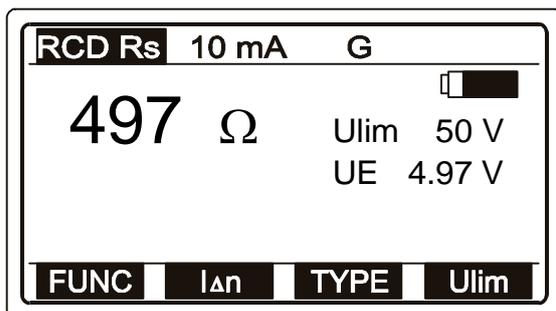
UE is displayed meaning auxiliary test probe has been used. In that case U<sub>c</sub> is measured with respect to auxiliary test probe (real ground) and present R<sub>s</sub> result is equal to Earth Resistance value.
