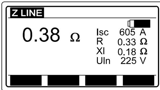
$$I_{psc} \text{ (Isc marked on display)} = \\ = U_n \cdot 1,06 / Z_{LINE}$$
