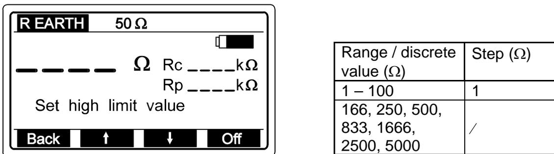
Fig. 24. Limit adjustment menu and table of presettable limit values
