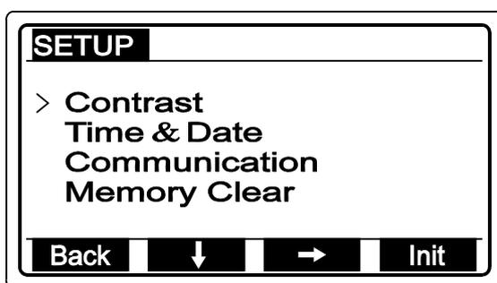
The **Init** key is production and service key only intended for inserting initial constants.
