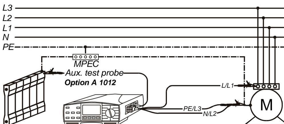
**Fig. 62.** Connection of Universal Test Cable and auxiliary test probe via optional Probe Test Lead (Order No. A 1012)
