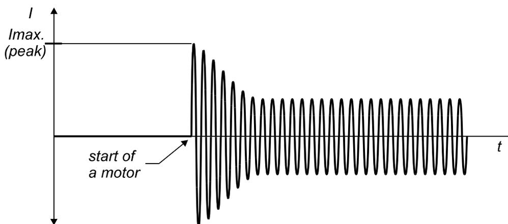
*Fig. 78. Motor's start up current*
