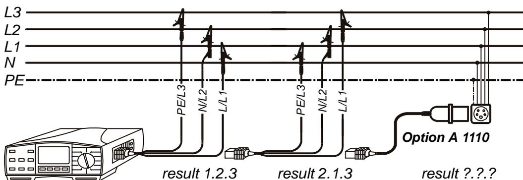
*Fig. 73. Connection of Universal Test Cable and optional Three-phase Cable (Order No. A 1110)*
