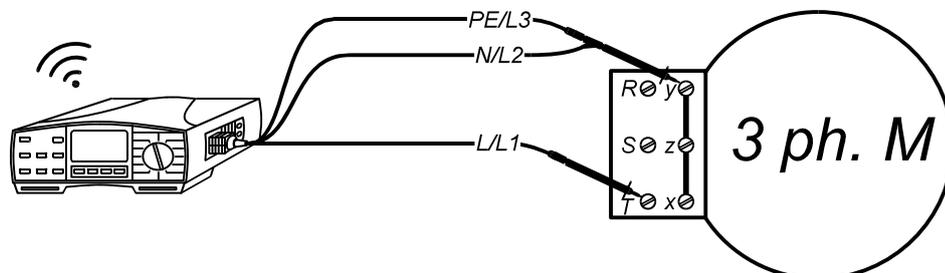
**Fig. 20.** Connection of Universal Test Cable
