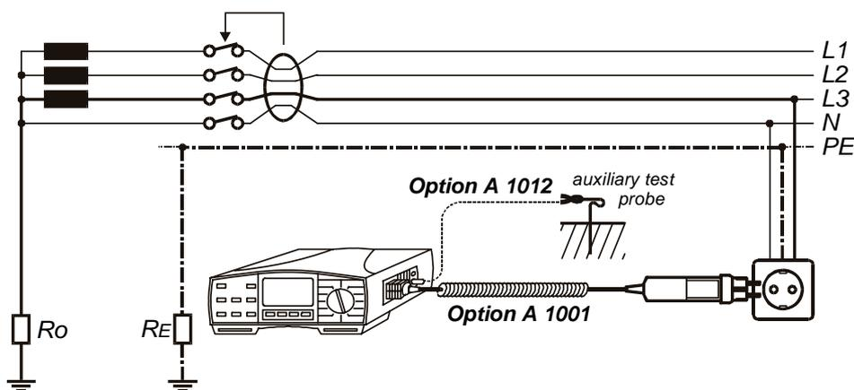
**Fig. 41.** Connection of optional Plug Commander (Order No. A 1001), measurement with or without auxiliary test probe connected via optional Probe Test Lead (Order No. A 1012)
