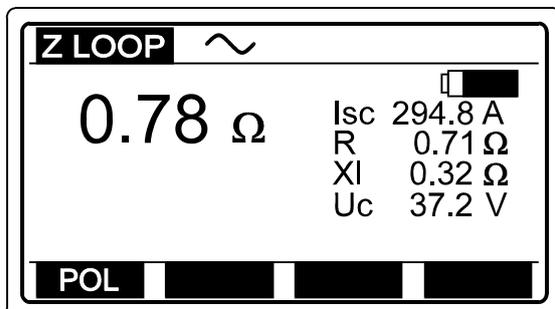
Uc..... Contact Voltage scaled to Prospective Short-circuit Current.
