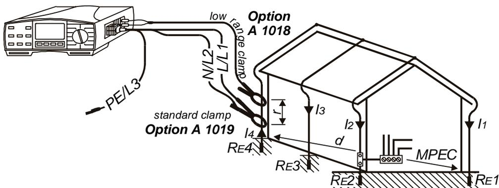
Fig. 32. Connection of optional Standard-range Current Clamp (Order No. A 1019) using Universal Test Cable and opt. Low-range Current Clamp (Order No. A 1018)
