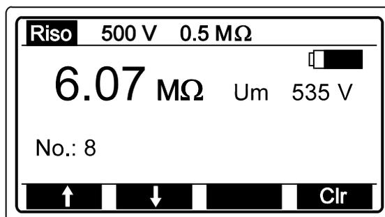
**Fig. 103.** Example of recalled last stored test result
