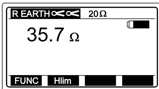
*Fig. 33. Example of Earth Resistance test result*
