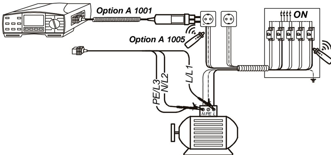
**Fig. 87.** Connection of Universal Test Cable or optional Plug Commander (Order No. A 1001) to energised installation
