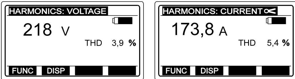
**Fig. 96.** Example of displayed result (THD and effective value of tested Voltage / Current)
