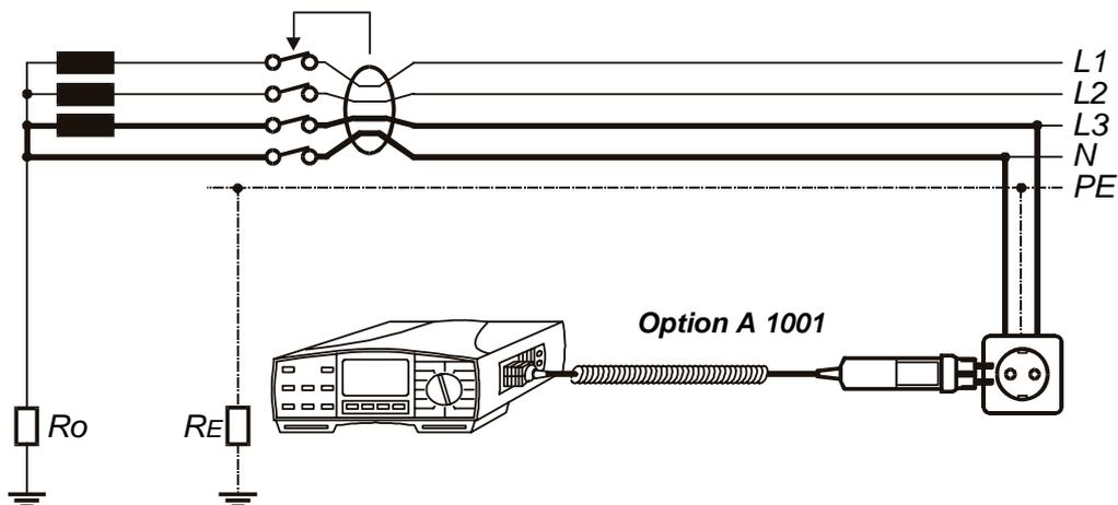
**Fig. 65.** Connection of optional Plug Commander (Order No. A 1001)
