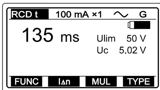
**Fig. 48.** Example of Trip out time test result
