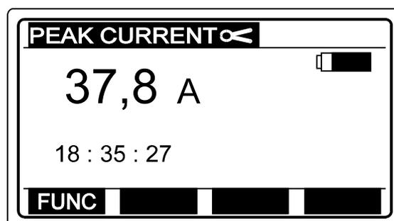
*Fig. 80. Maximal Peak Current value displayed*
