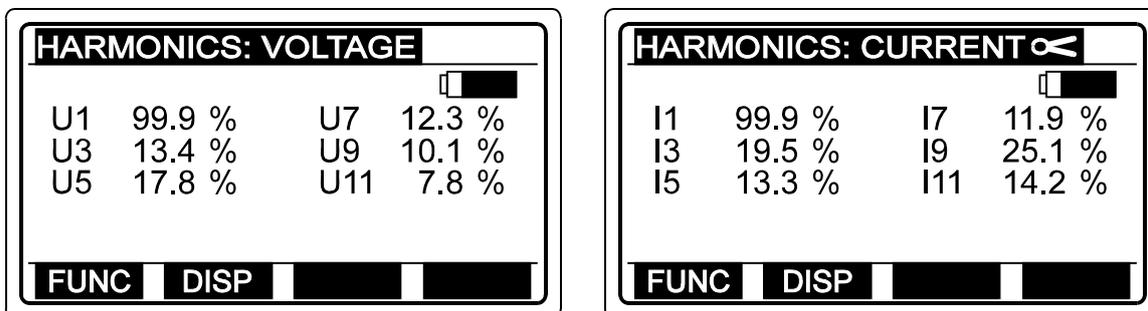
**Fig. 97.** Example of displayed result (individual harmonics from 1-st up to 11-th component)
