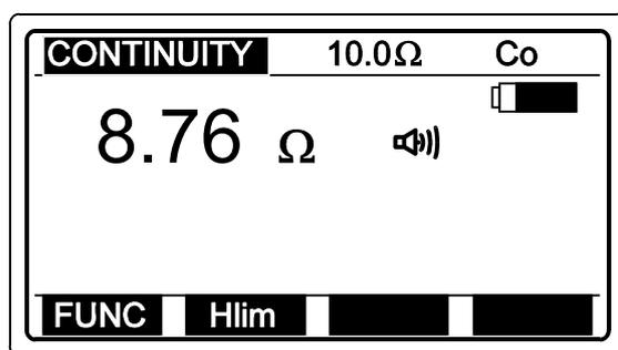
.....Displayed result is equipped with buzzer sign in case, if it is lower than set high limit value.
