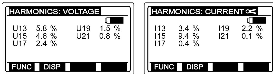
**Fig. 98.** Example of displayed result (individual harmonics from 13-th up to 21-th component)
