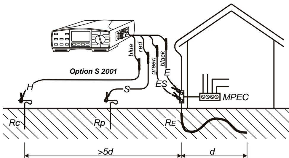
Fig. 25. Connection of optional Earth Test Set – 20 m (Order No. S 2001)
