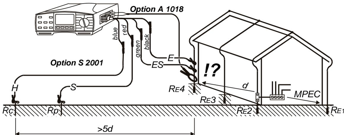
Fig. 29. Connection of optional Earth Test Set – 20 m (Order No. S 2001) and optional Low-range Current Clamp (Order No. A 1018)
