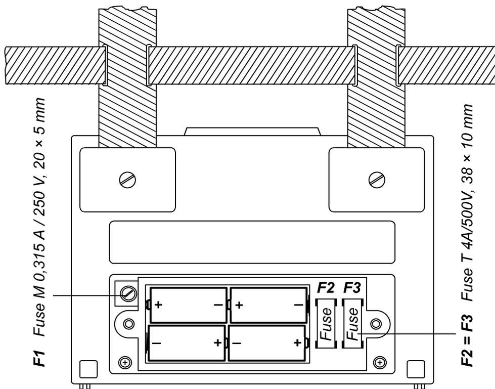
**Fig. 104.** Correct polarity of inserted batteries
