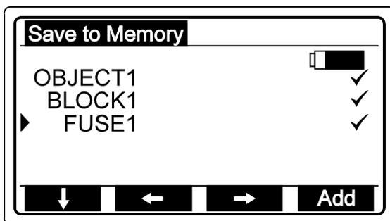
✓ .... All measurements attached (by means of PC SW only) to the measurement place are already carried out and results stored. Measurer can thus verify any time which measurements have not been done yet and where.
