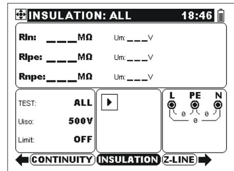
Figure 5.1: Insulation resistance
