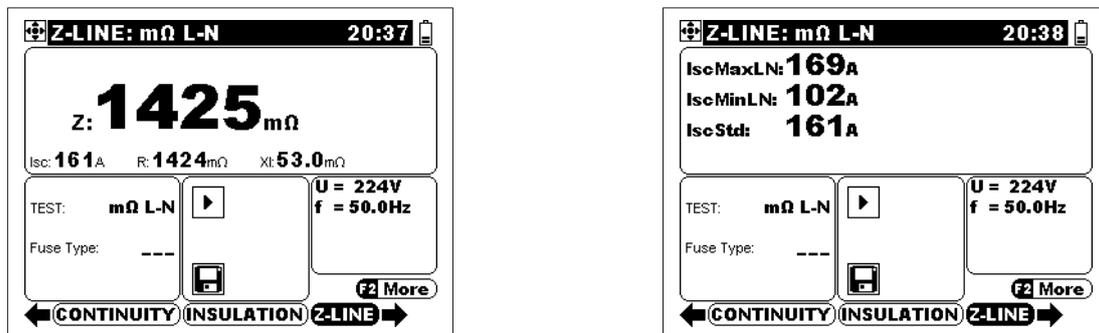
Figure 5.39: Example of 2 Ω line/loop measurement results
