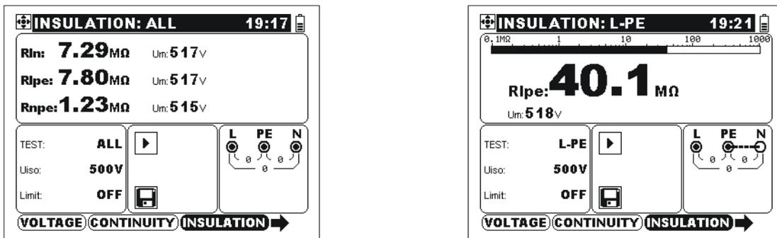
Figure 5.4: Examples of insulation resistance measurement results
