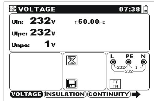
Figure 4.2: Example of typical Single test screen
