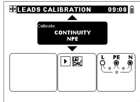
Figure 5.10: Test leads resistance compensation menu
