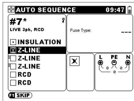
Figure 4.4: Waiting for right input condition to proceed
