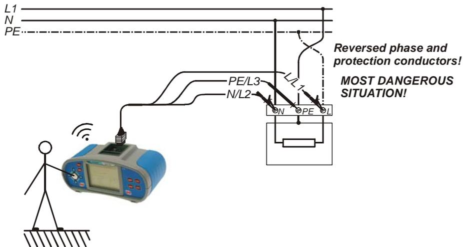
Figure 5.41: Reversed L and PE conductors (application of universal test cable)
