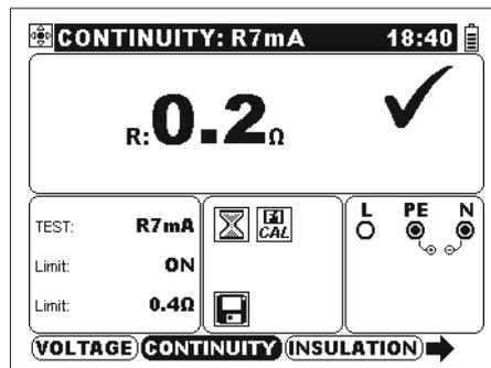
Figure 5.9: Example of 7 mA resistance measurement
