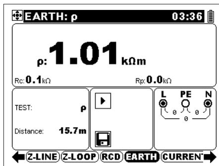
Figure 5.36: Example of specific earth resistance measurement result
