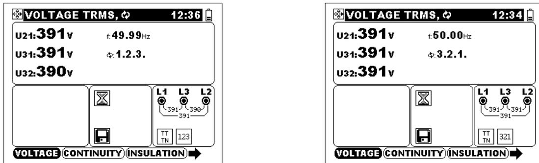
Figure 5.30: Examples of voltage measurement in three-phase system
