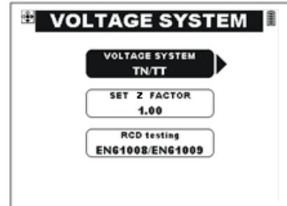
Figure 4.24: System parameters
