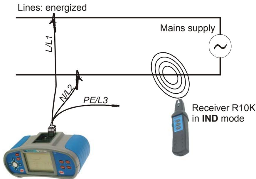
Figure C.3: The EurotestAT as a signal source for tracing lines
