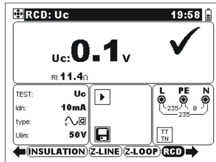
Figure 5.14: Example of contact voltage measurement results
