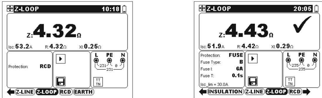
Figure 5.20: Examples of loop impedance measurement result
