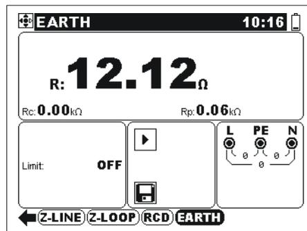
Figure 5.34: Example of resistance to earth measurement result
