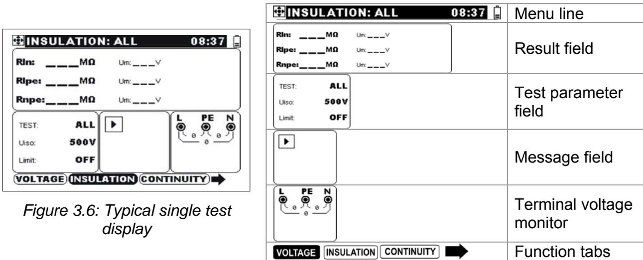
Figure 3.6: Typical single test display
