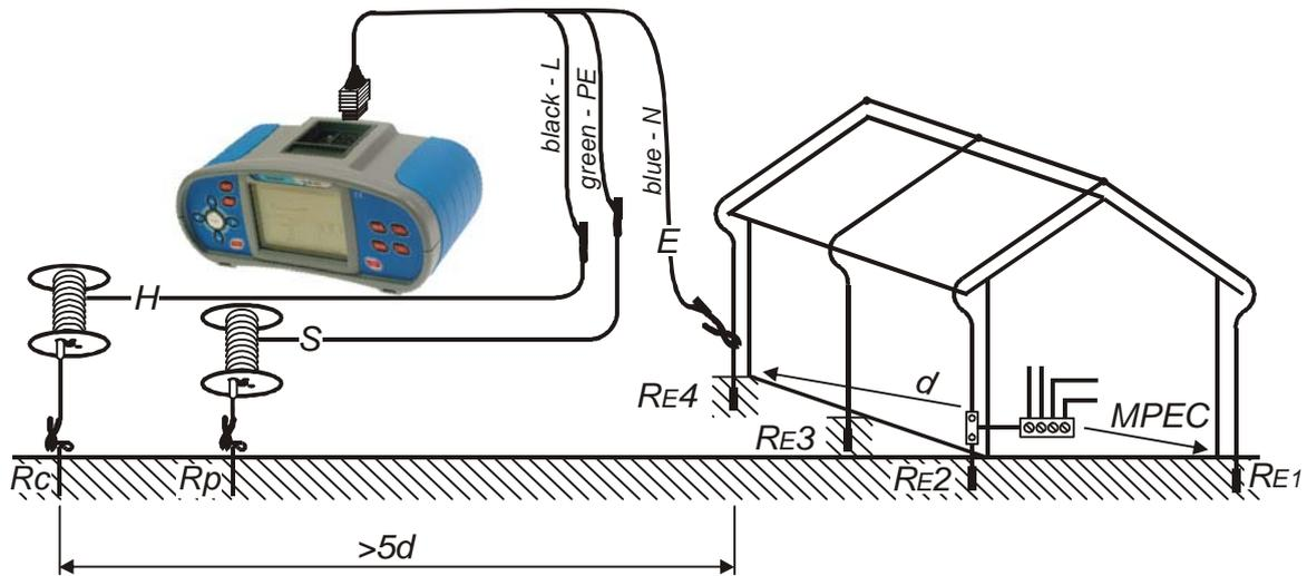
Figure 5.33: Resistance to earth measurement – lighting protection
