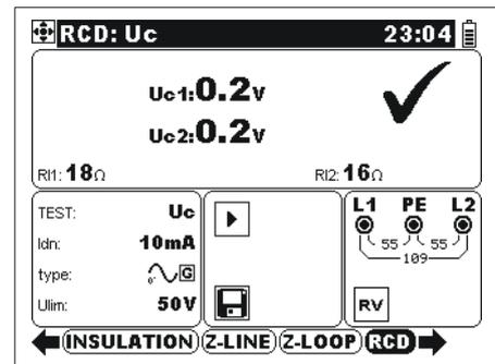
Figure E.3: RCD Uc test
