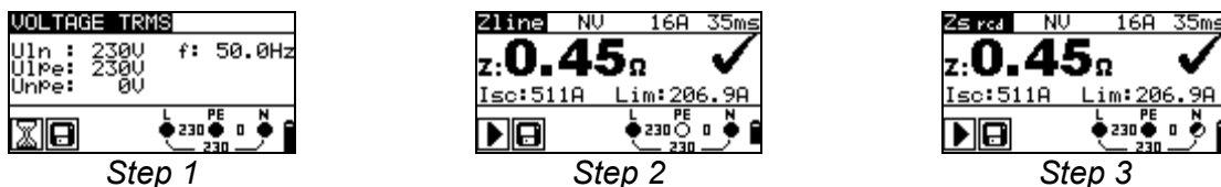
Figure 6.5: Individual steps of AUTO TT auto-sequence
