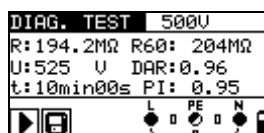
Figure 5.10: Example of PI and DAR diagnostic test results
