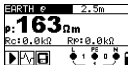
Figure 5.42: Example of specific earth resistance measurement result
