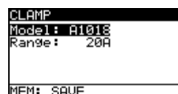
Figure 4.13: Configuration of current clamp measuring input
