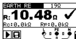
Figure 5.38: Example of earth resistance measurement result
