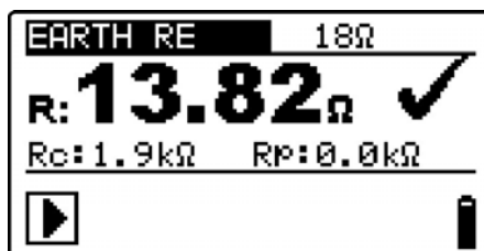
Figure 5.35: Example of earth resistance measurement result
